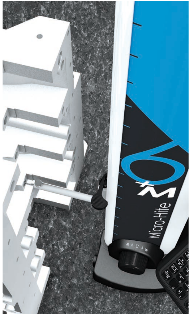
Measurement of an engine block
