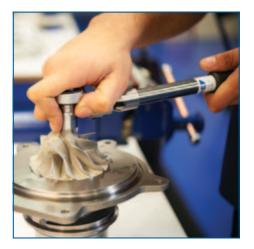
Improved accuracy, consistency and control. Accurate process control is ensured by reducing the risk of under and over tightening, due to unique Breaking Technology. This gives the operator more time to react once the target torque is reached
