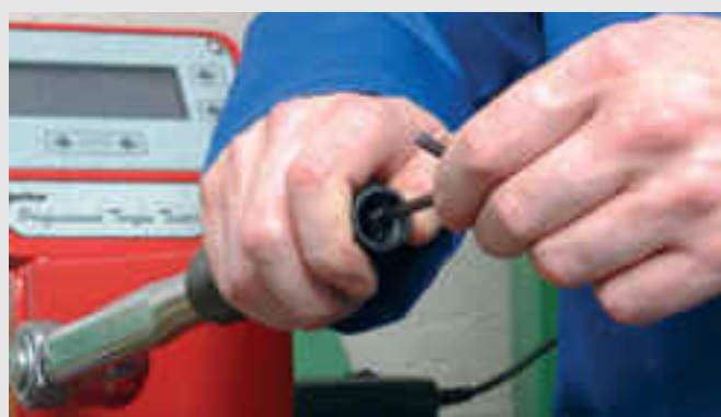
Setting a 'P' Type Torque Wrench
