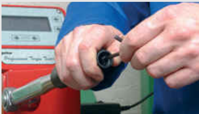
Setting a 'P' Type Torque Wrench
