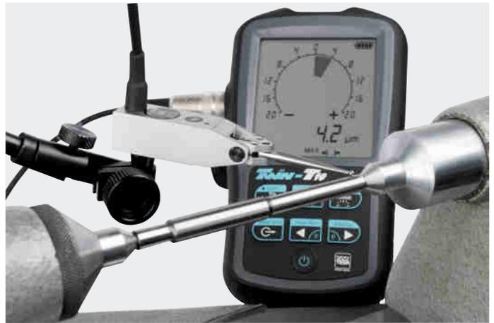
Run-out measurement with GT-31 lever probe
