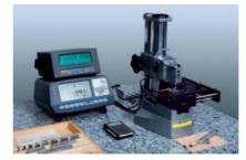
If specified, TESA can also provide the temperature device available as an option. This device has 4 PT100 platinum resistances, each capturing the temperature of the two gauge blocks along with that of both the measuring table and the support. Computeraided data processing lets you carry out any calibration most reliably and rationally – for sure.
