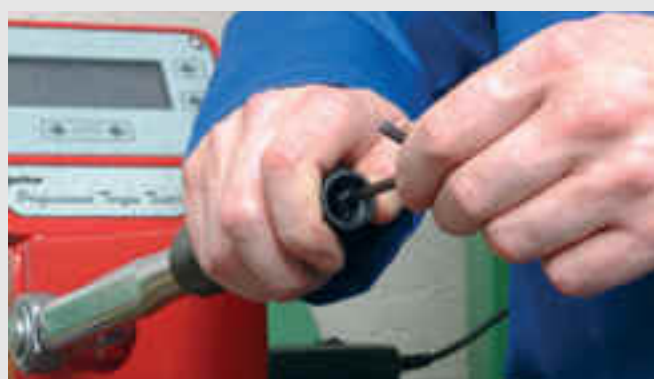
Setting a 'P' Type Torque Wrench
