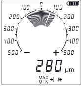
Measurement mode with MAX-MIN
