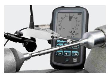
Run-out measurement with GT-31 lever probe
